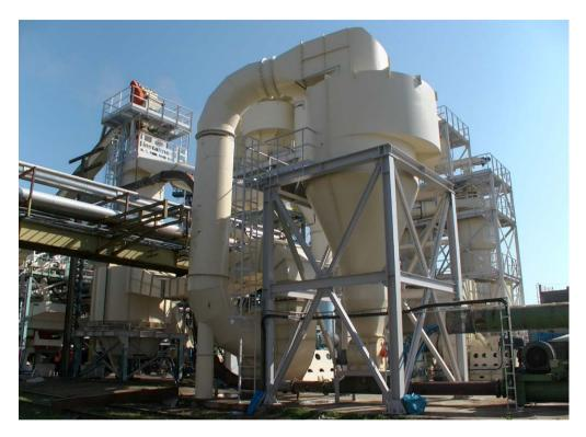
Its original design and revolutionary operating principle, developed and patent by Instalmec, gives the LPD cyclone incomparable benefits with respect to traditional cyclones. The main innovation is the special finned flow breaker system within the cyclone, which enables the separation of particles al lower air speed than in traditional cyclones.
