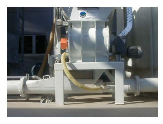
An increased use of recycled wood has raised the amount of silica contained in the wood dust, this generates serious problems of wear to the wood dust dosing and conveying machinery at the plant.
