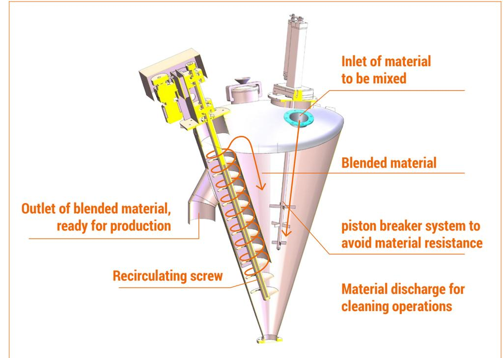
Blending occurs by means of a screw with constant/variable rotation. Part of the material inside the dosing mixer is extracted, whilst the remaining recirculates inside the cone.
